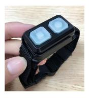
The two buttons are designated with symbols – a [] for Up, and a O for Down. To turn on the light hold the [] button in for 1.5 secs.
