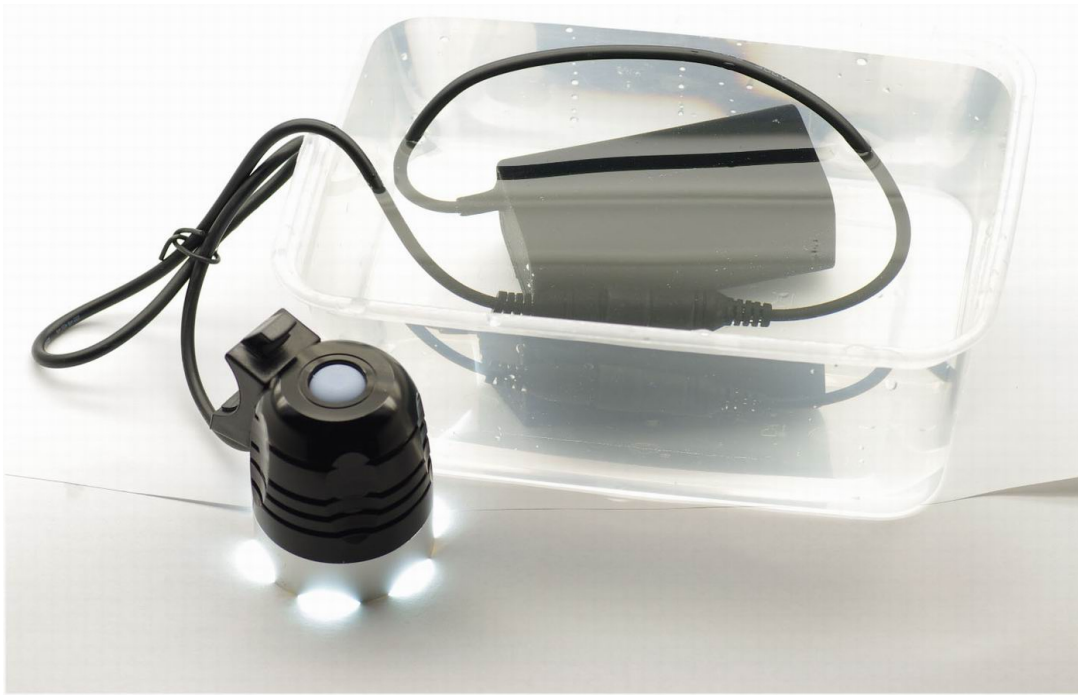
Illustration 1: Battery pack and connectors totally immersed, still powering C&B Seen 1000Lm lamp unit.....
